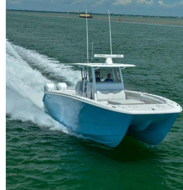
Performance Ranges: Cruise Speed: 40.8 - 49 mph / Cruise MPG: 1 - 1.2 mpg / Top Speed: 69 - 79 mph
