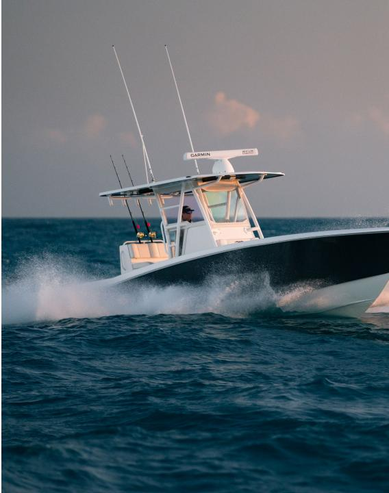
Performance Ranges: Cruise Speed: 29.8 – 52.9 mph / Cruise MPG: 1.4 – 1.8 mpg / Top Speed: 59.8 – 76.5 mph
